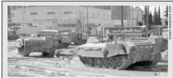
The chassis of the Achzarit infantry armored vehicle is built from Russian T-54/T-55 tanks captured in significant numbers by the Israel Defence Force. The chassis is completely rebuilt, with the 10-man crew and infantry compartment at the front and the new power pack at the rear. An additional layer of Israeli-developed passive armor is mounted on the chassis and the Achzarit has a combat loaded weight of 44 tons compared to the 36 tons of a turreted T-54/T-55. Infantry can enter and leave via hatches in the roof or the hydraulically operated clamshell door located in the right side of the vehicle.
